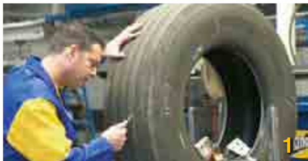
STEP 1 Initial inspection evaluates the safety of the casing
