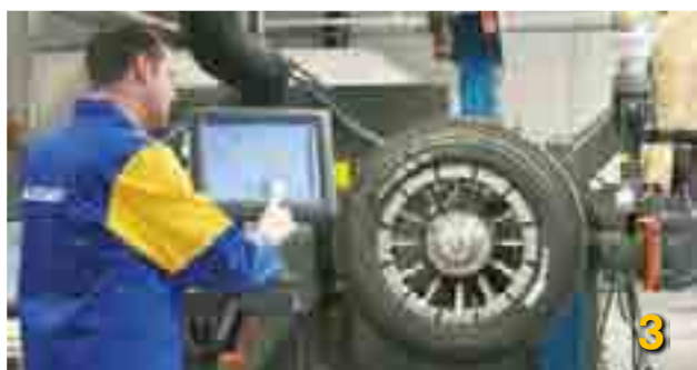
STEP 3 Buffing restores the tyre dimensions and a perfect balance
