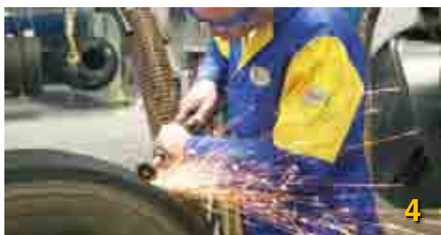
STEP 4 Skiving and filling repair and save valuable casings
